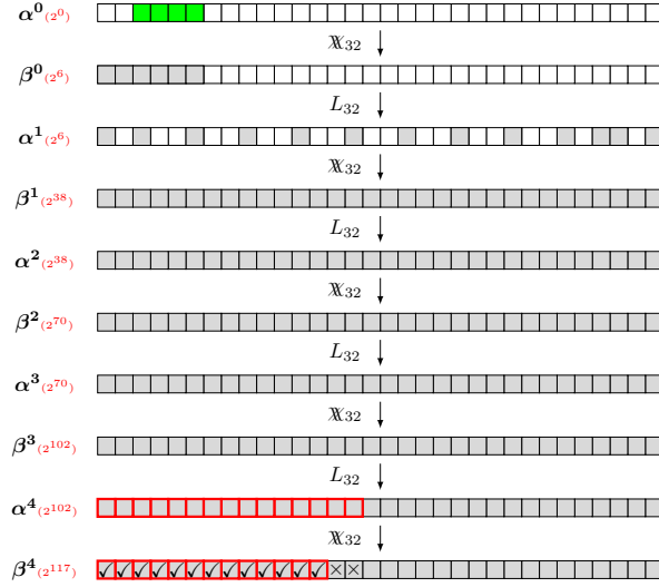
Fig. 17: The 4.5-round IP transition for ChiLow-32
