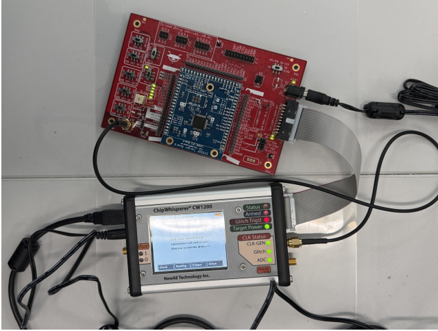
Figure 4: Experimental setup. A ChipWhisperer Pro connected to a STM32F415RGT6 target board.
