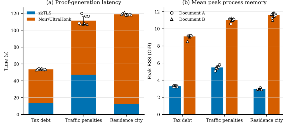
Fig. 7. Prover cost for the three evaluated profiles. Left: mean generation time split between fresh zkTLS generation and the Noir/UltraHonk stage, including its self-verification where points are session means and the whisker covers total-generation uncertainty. Right: mean peak RSS measured separately for the two sequential stages
