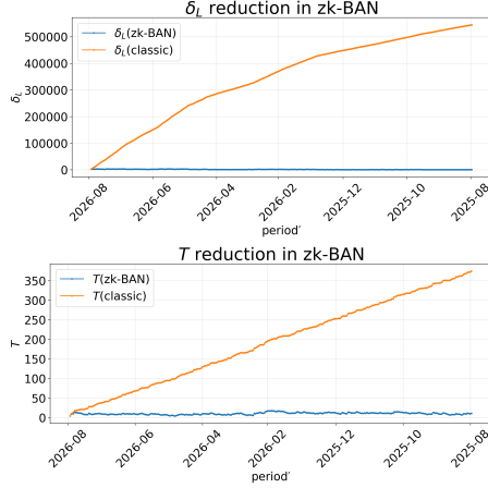
Figure 3: Comparison of \delta_L and T between classical signature based revocation and zk-BAN
